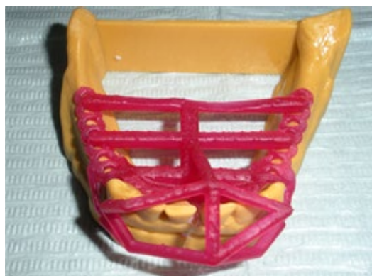
Figure:4 The 3D printed framework pattern on the 3D printed polyamide model
